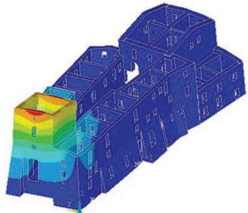
Figure 8. Mode 2 ( $f = 6.50 \text{ Hz}$ ).
