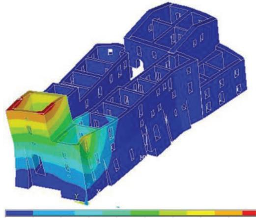
Figure 7. Mode 1 ( $f = 5.73 \text{ Hz}$ ).
