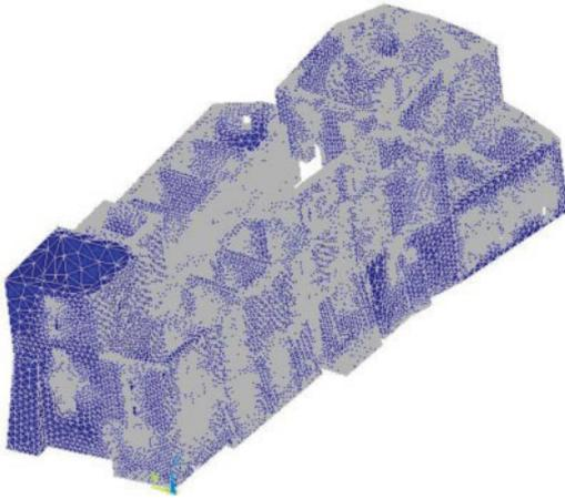
Figure 6. Mesh with solid elements.
