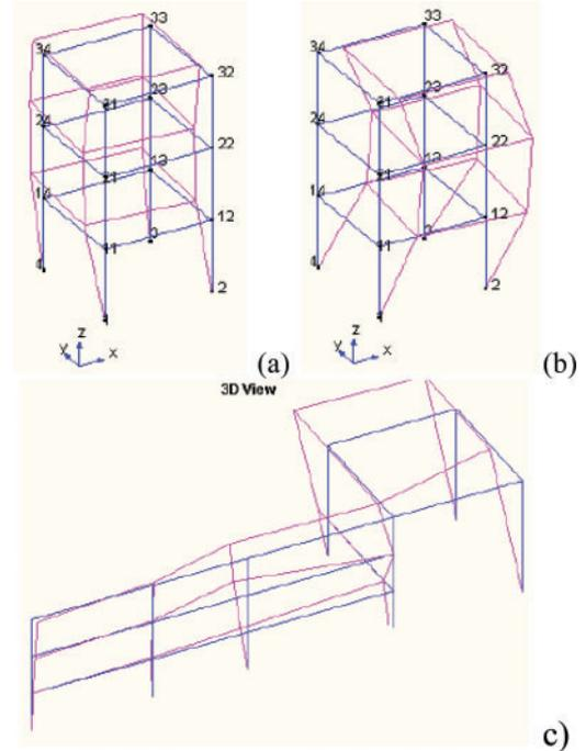
Figure 5. Experimental modal shapes with accelerometric data: (a)  $f = 5.6$  Hz (Translational Y Tower), (b)  $f = 6.7$  Hz (Translational X Tower), (c)  $f = 6.2$  Hz (Translational Y building B).
